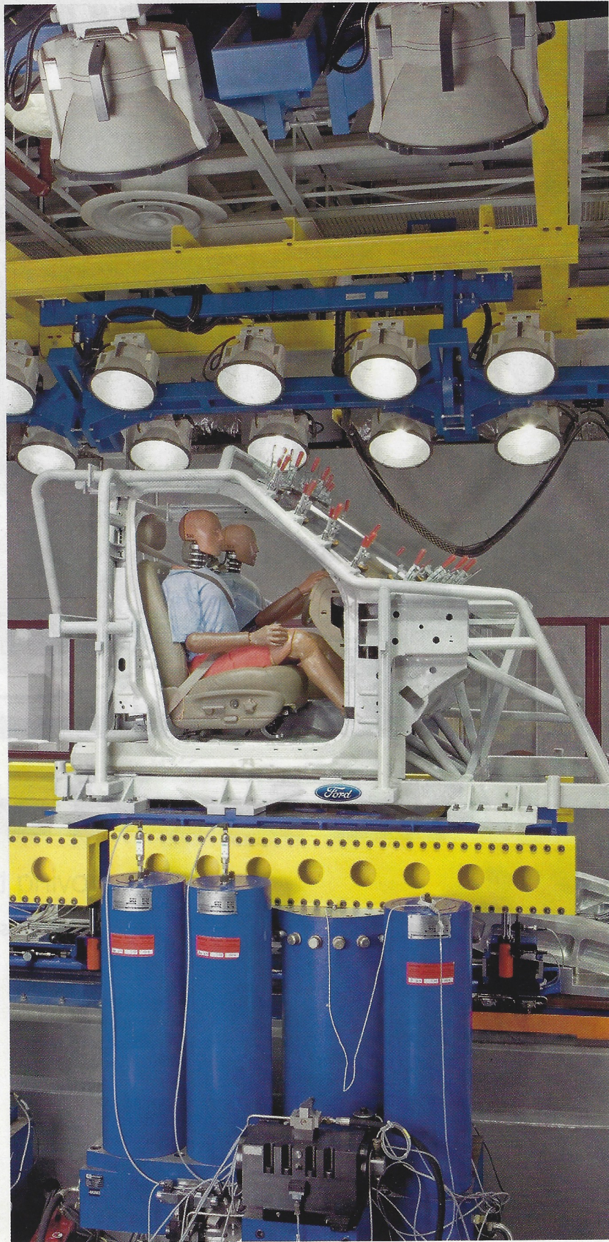
ABOVE: This Servo-Hydraulic Reverse Crash Simulator studies full-vehicle collisions including pitching and nonpitching modes, rear crashes, and side impacts.
