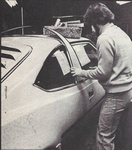
Motortown employe installs roof band on Hornet.
