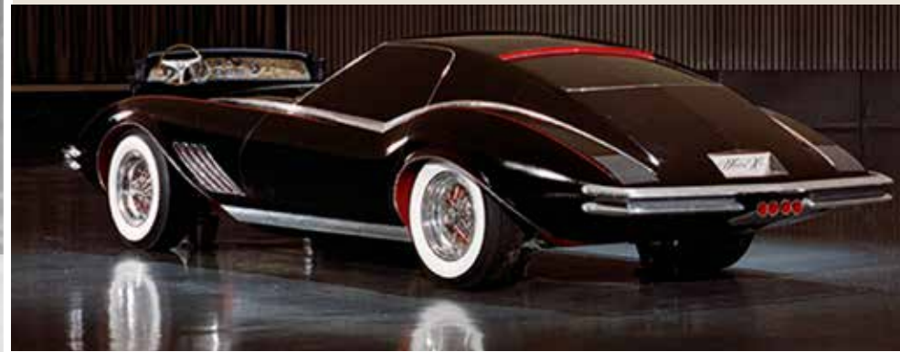
1958-'62 XP-700 Corvette Phantom: At Mitchell's direction, designer Ed Wayne customized a 1958 Corvette with a Ferrari-inspired elliptical grille, Dayton wire wheels, side pipes, air scoops, and a tail that previewed the '61 production model. It traveled the 1959 show-car circuit, Mitchell drove it on the road, and it reappeared in 1960 with further modifications, including a "double-bubble" Plexiglas top with a
