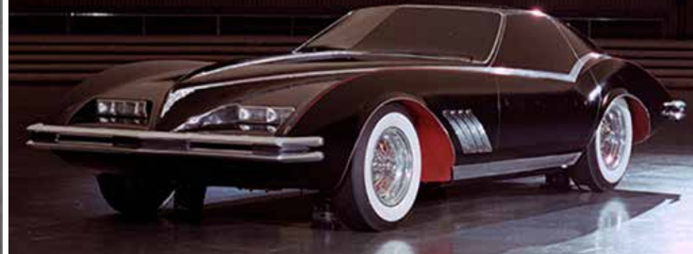
1958-'62 XP-700 Corvette Phantom: At Mitchell's direction, designer Ed Wayne customized a 1958 Corvette with a Ferrari-inspired elliptical grille, Dayton wire wheels, side pipes, air scoops, and a tail that previewed the '61 production model. It traveled the 1959 show-car circuit, Mitchell drove it on the road, and it reappeared in 1960 with further modifications, including a "double-bubble" Plexiglas top with a
