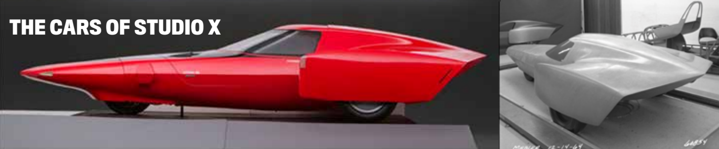
1964-'69 XP-800 Astro III: Designed by Lonberger and Studio X head Bob Larson and powered by a GM Allison gas turbine, the Astro III was just hip-high, its pointed nose on tandem tires that looked like a single front wheel, its canopy powered up and forward. “It had been an ongoing project for a year,” Lonberger recalled in a 2011 Dean’s Garage interview, “but did not have the aircraft look that Mr. Mitchell wanted. So we turned it from a three-lump collection of elliptical
