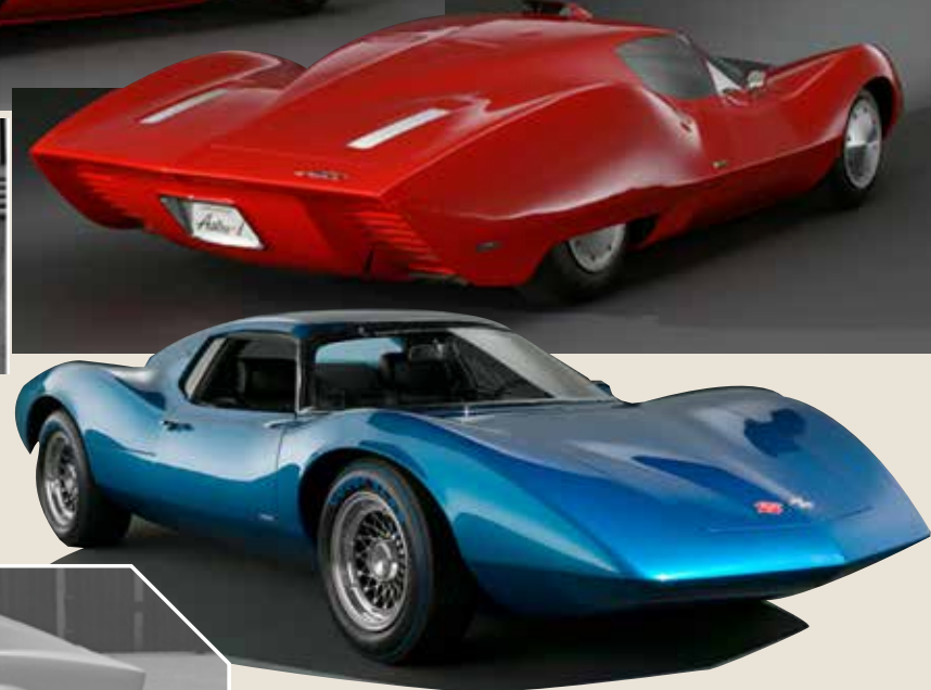
1966-'68 XP-880 Astro II: This curvacious drivable mid-engine exploration was much less radical than Astro I. Designed by Shinoda, Lonberger, Dave Clark, and Chuck Jordan, its suspension was (Corvette) transverse leaf-spring, and its rear section was raised for access to its mid-mounted V-8 and modest cargo space.
