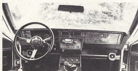
Useful but unsightly Concord/Spirit/Eagle underdash shelf and hard-to-see gauges.
