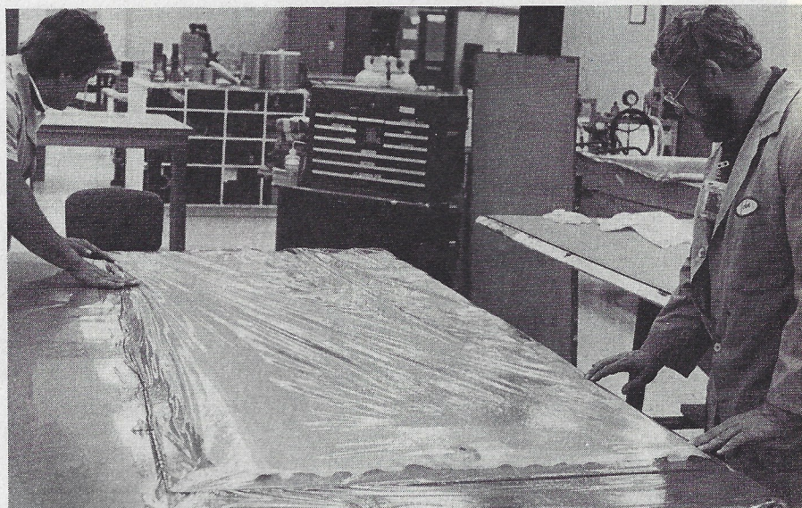
Ford engineers prepare one of many carbon fiber/Nomex honeycomb composite panels that make up the Mustang GTP tub.
