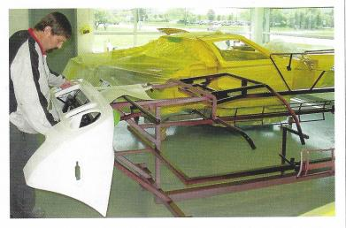
The Ford GT does a lot of traveling before it gets an engine or gearbox. Even when it is assembled and arrives at Saleen Special Vehicles, it is disassembled for paint and prep before going back onto a truck for more traveling. We were surprised at the care and quality-control-detailing accomplished before the body/chassis goes off to have the drive line installed — very carefully.
