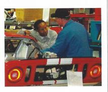
where an assembly book is tied to each vehicle, then they go through our paint system, then they're walked through the line." The remainder of the outer body—hood, front and rear fascias and lower side "doglegs"—are composite. The fenders and hood get painted on the body, while the other composite parts go through the process on a rack directly behind the vehicle.
