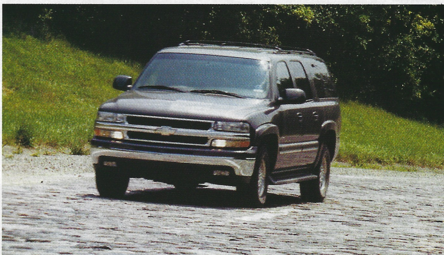
A Ford engineer (top) checks the sleekness of a Mustang convertible inside the "world's quietest aeroacoustic wind tunnel" at the Driveability Test Facility in Allen Park, Mich. A drive over the Belgian Blocks (bottom) at GM's Milford test facility accelerate suspension wear in real time.
