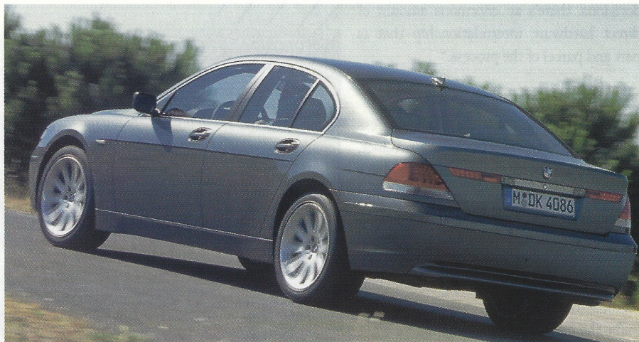
BMW's Chris Bangle took a lot of heat for the design of the new 7 Series. He admits that a lot of the controversial shapes were driven by the size and shape of the new V-8 engine, crash structure and roomier interior package.
