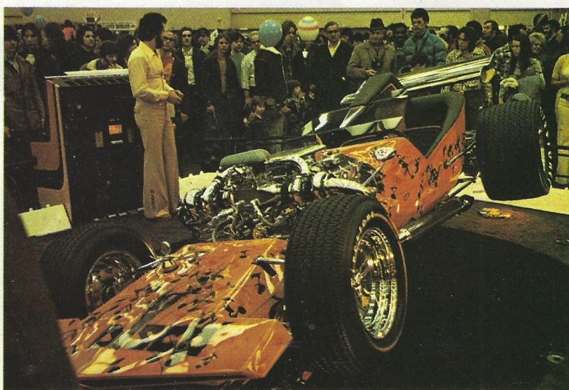
This beautiful racer-like winged "Disco" is based on a '25 Ford and gets its power from a glistening turbocharged '69 Chevy 409 bored to 440 cubes.
