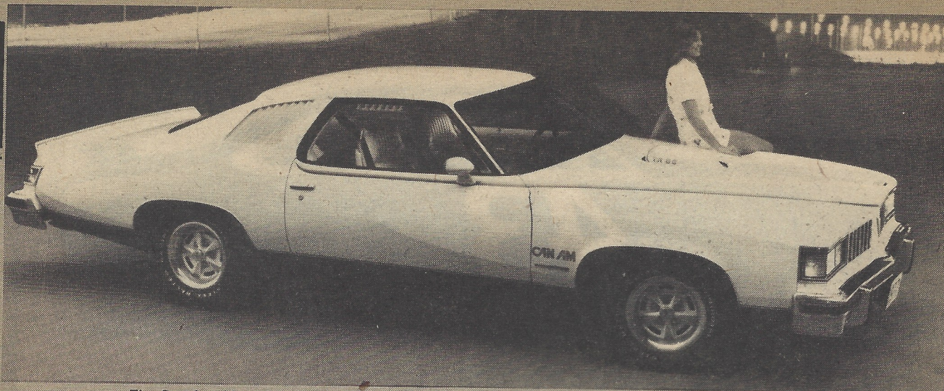
The Can Am, Motortown's idea of what a LeMans Sport Coupe should be, complete with 400-cube V8, RTS suspension with front and rear stabilizer bars and, of course, stripes and hood scoop.
